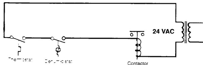
In the series circuit, both the temperature and relative humidity need to be at or above the settings of the controls to activate the air conditioner.
