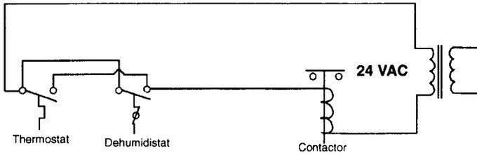
In the parallel circuit, the air conditioning can be activated by either temperature or relative humidity.
